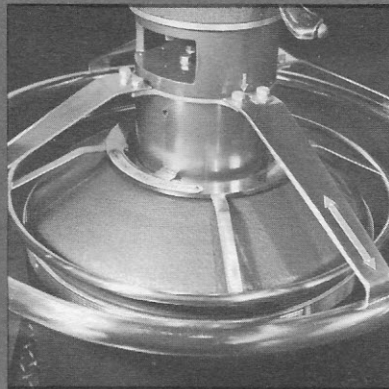
Arrows on steering wheel show direction of wheels. Lower ring locks column and controls drag.
