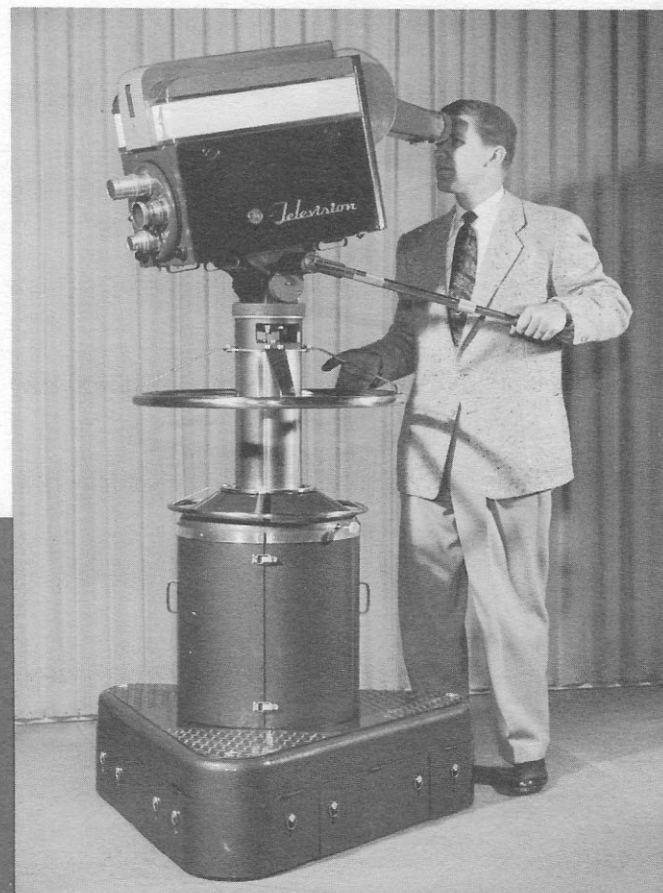
Counterbalanced camera is easily raised or lowered by light pressure on steering wheel.
